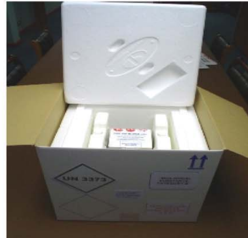
8. Place specimen box in the centre of the thermal unit and between the two Cool-Packs. Place lid and fold over all the outer flaps.
