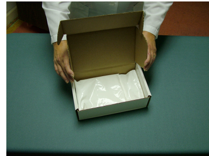
Gel wraps should fully cover 95kPa bag.
