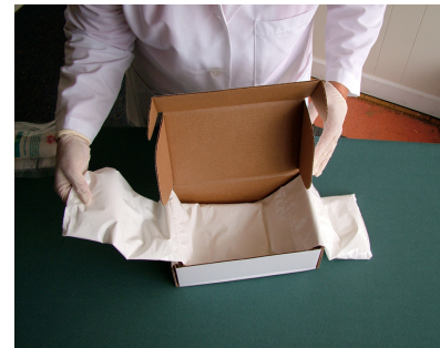
Place 2nd gel pack over 1st gel wrap..
