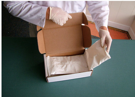
Fold one gel wrap over 95kPa bag.
