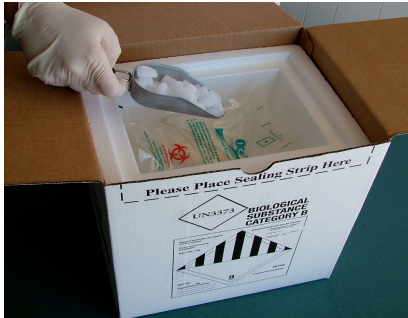
Place 4.0 lbs (1.82 kg) of dry ice on top.
